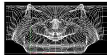
Cylindrical Projection produces UVs that are overlapping and distorted in this example
