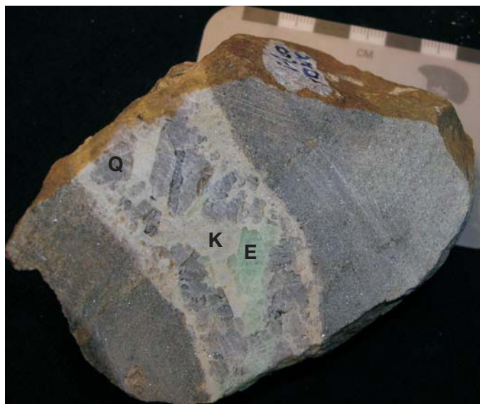
FIG. 4. Emerald-bearing pegmatitic vein comprised of quartz (Q), potassic feldspar (K), and emerald (E). The host rock is a foliated phlogopite schist of the Proterozoic Saxi unit. The minerals within the vein show no evidence of deformation, while the biotite in the host rock defines a vein-parallel foliation. Specimen DYK06-007.
