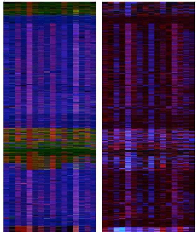
**Figure 7.** Spectral fingerprints for the *Breaks* track “Blowout”, with Bark analysis, left, and Flux/Centroid/Roll-off, right. The section changes are clearly displayed: in this track, both low and high frequencies are removed during the breakdown, leaving primarily the midrange, shown green in the Bark analysis.
