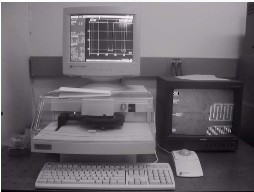
Fig. 43 Schematic drawing of a surface profilometer. Courtesy of Sloan Technology Corporation
