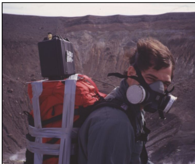
Fig. 4. A walking traverse with a backpack-mounted FLYSPEC at Vulcano, Italy, 2002.
