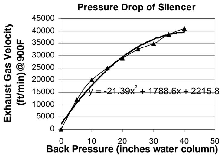
Figure 8 Modeled Relation between Back Pressure and Gas Velocity.
