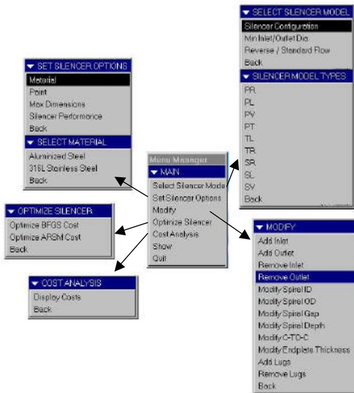
Figure 10 Menu structure of the program developed with Pro/Toolkit.
