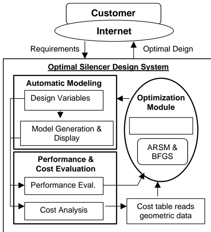
Figure 1 Structure and information flow for the optimal silencer design system.
