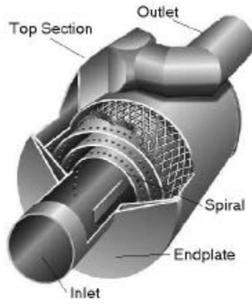
Figure 3 Basic configuration of an industrial silencer [15].
