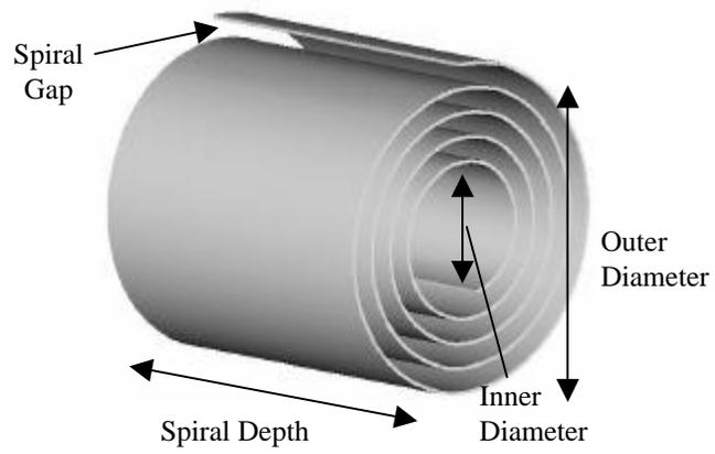
Figure 4 Geometric parameters of the spiral.
