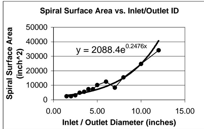
Figure 7 Relation between inlet / outlet diameter and the damping surface area from existing designs.
