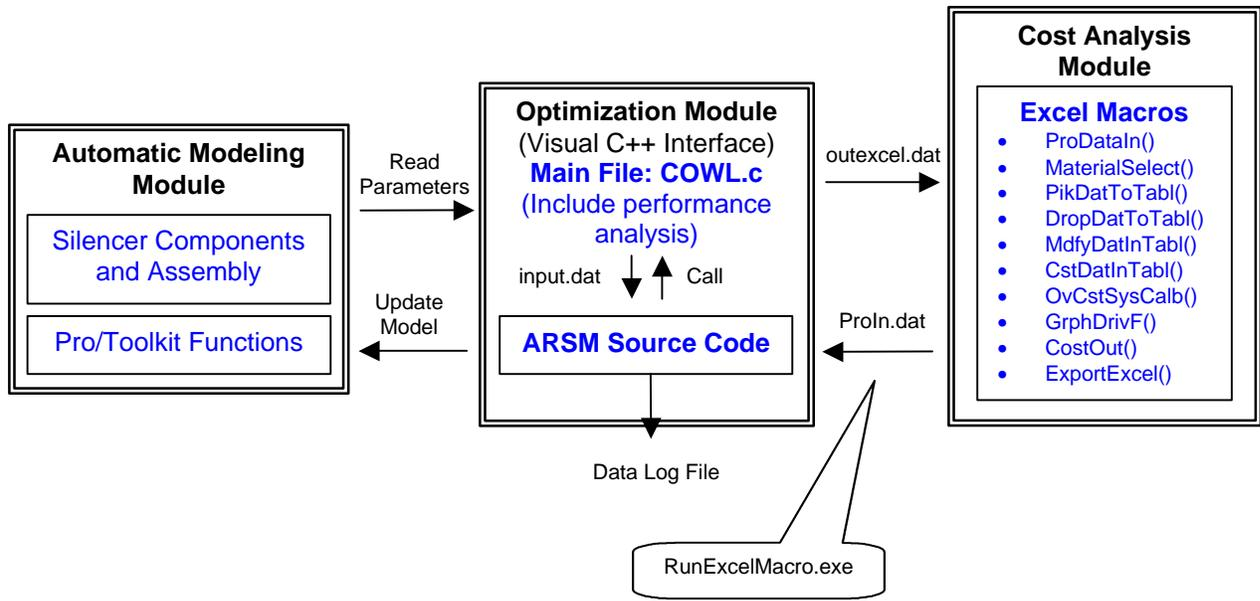
Figure 9 Interactions between system modules.
