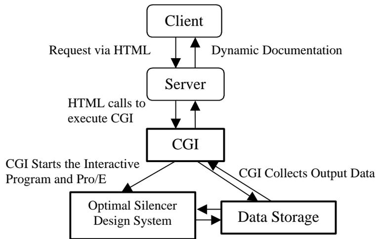
Figure 11 Information flow between the web application and the silencer design system.
