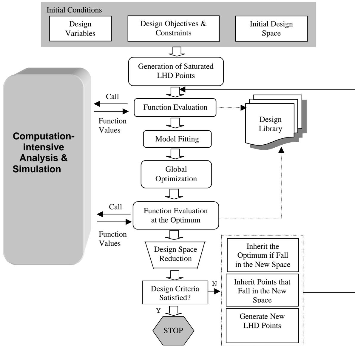
Figure 2 The flowchart of the ARSM.
