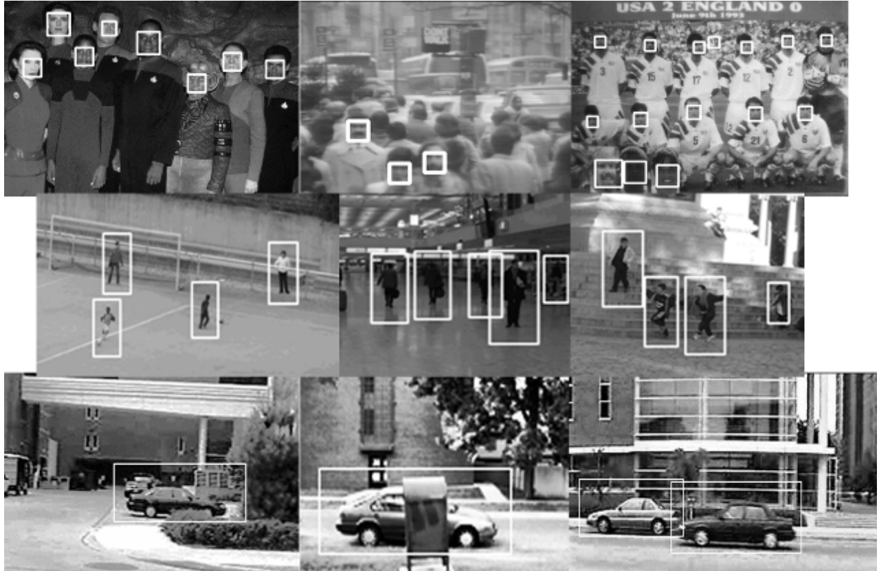
Fig. 11. Detection results. First row – CMU face dataset. Second row – INRIA pedestrian dataset. Third row – UIUC car dataset
