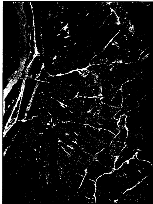
Figure 34. Aerial photograph showing 1983 debris flows in vicinity of Wahleach Power Station (circled) in the Fraser Valley. Multiple starting points of debris flows are arrowed. Note at least three sources for the debris flow in Ted Creek (A) discussed in text. Point "D", located just south of Ted Creek, is an area of topographic linears associated with rock slope deformation illustrated in Figure 19. (BC 83020-104)
