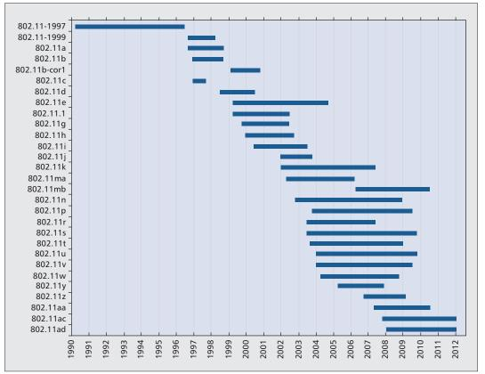
With the increasing size of areas covered by WLANs, specifying a network management standard has become urgent. The 802.11k and 802.11v amendments provide a framework for radio resource and network management, respectively.
