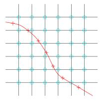
Figure 2: The fluid grid points ( $\circ$ ) and moving fiber mesh points (+).
