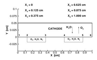
Figure 2: Computational domain, consisting of a 2D slice through the cathode over a pair of flow channels.
