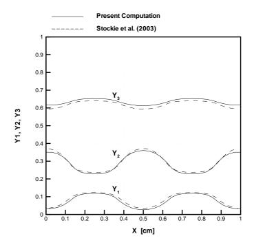
Figure 4: Comparison of computed mole fractions at the catalyst boundary (the top boundary) for species  $(1, 2, 3) = (O_2, H_2O, N_2)$ .
