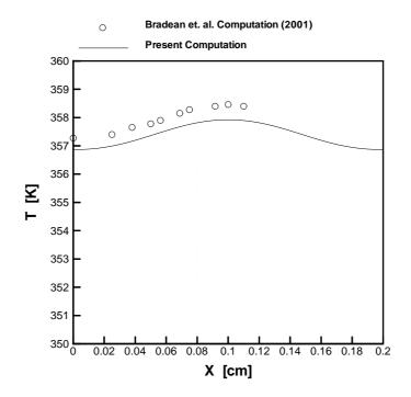
Figure 7: Comparison of temperature distribution at the catalyst boundary (the top boundary) with the results of Bradean et al. (2001).
