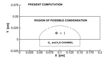
Figure 8: Region of possible condensation predicted by the present two-species non-isothermal computation with one channel.
