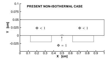
Figure 11: Region of possible condensation predicted by the present three-species non-isothermal computation with two channel.
