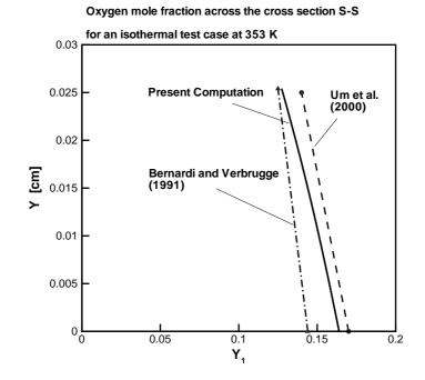
Figure 10: Comparison of oxygen mole fraction  $(Y_1)$  across the porous media of cathode, at the cross-section S-S of the previous figure.
