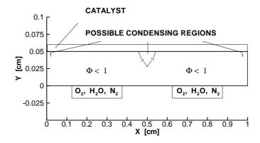
Figure 5: Regions of possible condensation predicted by the model, assuming isothermal conditions.
