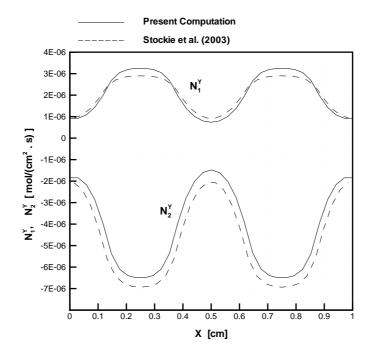
Figure 3: Comparison of molar fluxes at the catalyst boundary (the top boundary) for species  $(1, 2) = (O_2, H_2O)$ .
