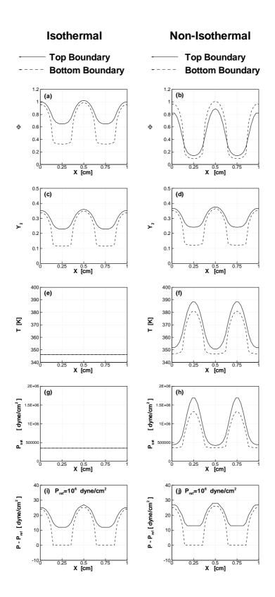
Figure 12: Comparison of three-species isothermal (left) and non-isothermal (right) computations.
