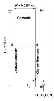
Figure 9: Cathode and channel schematics in Um et al. (2000) computation.
