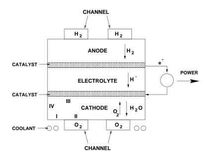
Figure 1: A schematic picture of a proton exchange membrane (PEM) fuel cell.
