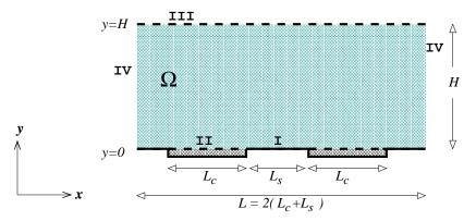
Figure 2. Dimensions of the model domain  $\Omega$ : GDL thickness H, channel width  $L_c$ , separation distance  $L_s$ , and total width  $L = 2(L_c + L_s)$ . The boundary components are identified by Roman numerals I-IV.
