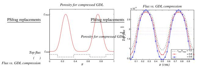
Figure 12. Variable porosity simulations use a porosity that varies in the *x*-direction as pictured on the left, with the channels shown for comparison. The flux profiles corresponding to porosity ratios of  $\varepsilon_{min}/\varepsilon_{max} = 1.0, 0.8$  and 0.6 are shown in the plot on the right.
