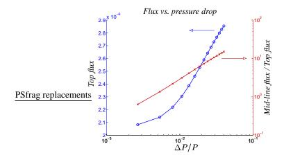
Figure 10. Variations in the membrane reactant flux and the midline-to-top flux ratio versus pressure drop.
