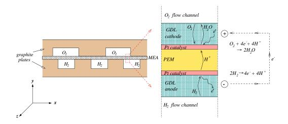
Figure 1. A proton exchange membrane fuel cell and its component parts. On the left is a cross-sectional view of the cell, showing the MEA sandwiched between the oxygen and hydrogen flow channels. The in-channel gas flow is directed normal to the page. On the right is a close-up view of the MEA. The reaction occurring at each electrode is listed on the far right, along with the flow of electrons generated when the anode and cathode are linked in an external circuit.
