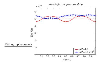
Figure 13. Reactant mole fraction (left) and total reactant flux at the membrane (right) for the anode.
