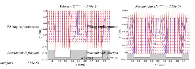
Figure 6. Vector plots of velocity and total flux for the cathode "base case." The velocity and flux streamlines are superimposed on the vector plots to highlight the flow direction. The locations of the flow channels and landing areas are indicated by the shaded regions.
