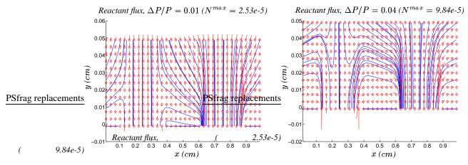
Figure 8. Vector plots of the total flux for two values of the channel pressure drop.
