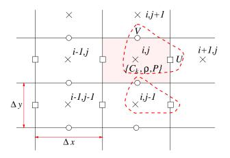
Figure 3. A picture of the grid used to discretize the problem, with the placement of unknowns indicated in a cell: "×" for P,  $\rho$  and  $C_k$ ; " $\circ$ " for V and  $J^y$ ; and " $\square$ " for U and  $J^x$ . The dashed line encloses those points which are labeled with the subscript i, j.
