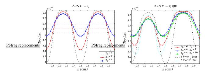
Figure 11. Variation in the membrane reactant flux for various levels of anisotropy in the transport coefficients. The results in the left figure are for a zero channel pressure difference. The right figure corresponds to  $\Delta P/P = 0.001$  which, while nonzero, is still small in comparison with the simulations in Sec. 4.4. The isotropic results for  $\Delta P/P = 0$  and 0.01 are shown as dotted lines for comparison.
