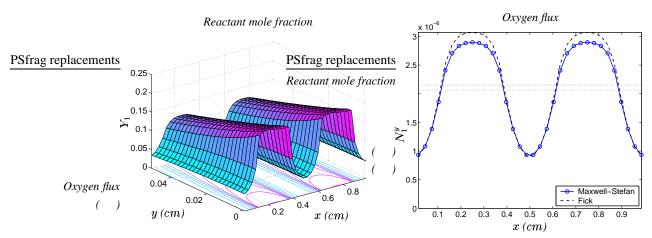
Figure 5. Reactant mole fraction (left) and total reactant flux at the membrane (right) for the cathode "base case."
