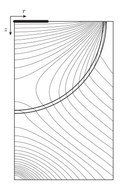
Figure 1.10: Illustrated is the temperature profile of the crucible and the holder. Note the cold spot at the base of the holder at r = 0. This pattern is expected to persist in the presence of the convective flow of the melt since in Section 1.8 it is shown that the fluid flow is essentially inviscid.
