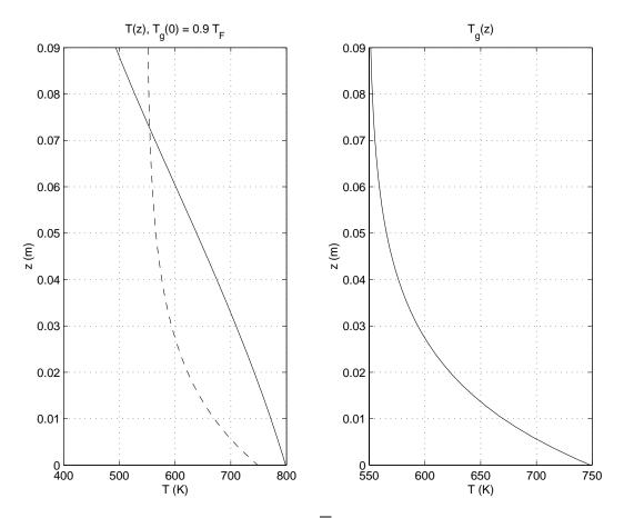
Figure 1.3: The left graph shows the average temperature  $\overline{T}(z)$  over the length of the crystal with the temperature of the gas  $T_g(z)$  overlaid for comparison. On the right is just the temperature of the gas. The uniform interface velocity is  $v_p = 70$  mm hr<sup>-1</sup> and the deviation from uniform,  $\partial S/\partial t - v_p = -29.6$  mm hr<sup>-1</sup>.
