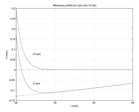
Figure 1.12: Menisucus profile for the melt/gas interface,  $f_l(r,t)$  for no rotation and at 10 rpm.
