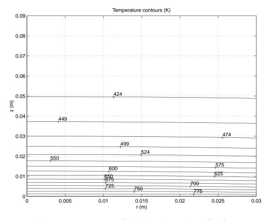
Figure 1.5: Temperature profile T(r, z) in the crystal with  $\delta = 1/3$ .
