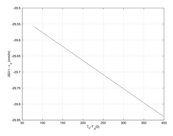
Figure 1.4: The deviation from uniform interface velocity,  $\partial S/\partial t - v_p$ , as a function of  $T_F - T_q(0)$ .
