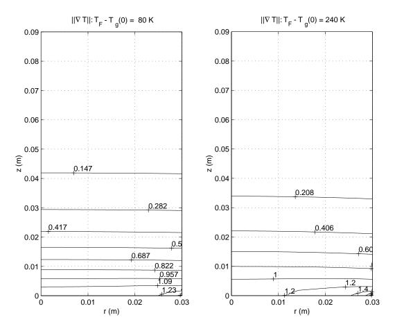
Figure 1.7: Norm of the gradient of the temperature as  $T_g(0)$  varies. The figure on the left has  $T_g(0) = 720$  K and the figure on the right has  $T_g(0) = 560$  K.
