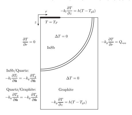
Figure 1.9: Shown here is the geometry and boundary conditions for solving the steady state heat equation in the crucible and the holder. Summarizing the parameters:  $k_l = 9.23 \text{ W m}^{-1}\text{K}^{-1}$ ,  $k_q = 1.5 \text{ W m}^{-1}\text{K}^{-1}$ ,  $k_g = 120 \text{ W m}^{-1}\text{K}^{-1}$ ,  $T_F = 798.4 \text{ K}$ ,  $Q_{\text{app}} = 1200 \text{ W}$ ,  $h = 10 \text{ W m}^{-2}\text{K}^{-1}$ ,  $T_{g1} = 600 \text{ K}$ ,  $T_{g2} = 700 \text{ K}$ , and  $t_r = 0.03 \text{ m}$ .
