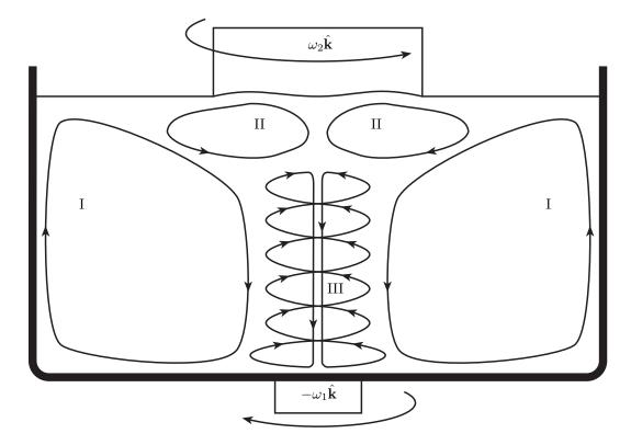
Figure 1.11: Experimentally observed flow pattern of the liquid InSb. The three major features are I: a buoyancy drive cell; II: a cell driven by Ekman pumping; III: a transient spiral.
