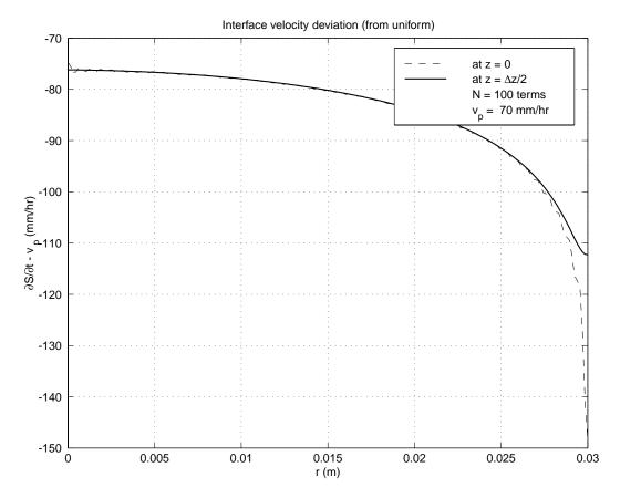
Figure 1.6: Radial dependence of the relative speed of the interface  $\partial S/\partial z - v_p$  with  $\delta = 1/3$ . The dashed curve is the speed at z=0 while the solid curve is the speed just inside the interface at  $z=\Delta z/2$ . Negative values indicate that the interface is growing downwards. Finally, the N=100 indicates that the Bessel series solution was truncated at 100 terms.
