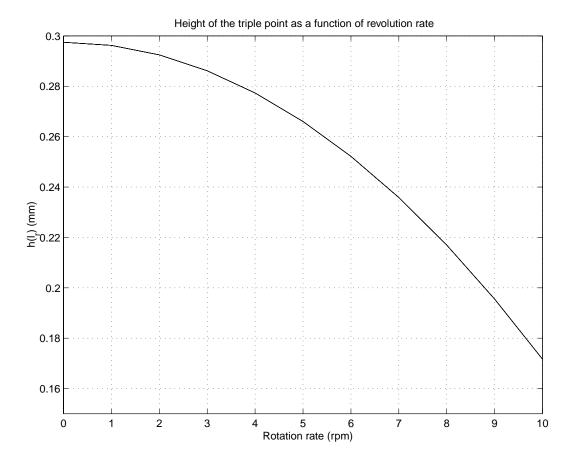
Figure 1.13: Position of the triple point as a function of the rotation rate.
