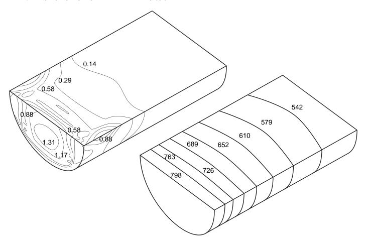
Figure 1.8: von Mises stress of an InSb crystal together with the corresponding temperature distribution.
