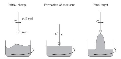
Figure 1.1: The Czochralski crystal pulling technique.
