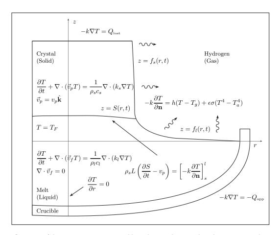
Figure 1.2: Summary of the equations, geometry and boundary conditions. The z direction is greatly exaggerated for clarity in that the interface z = S(r, t) is shown in Section 1.9 to lie very close to the line z = 0. See Section 1.7 for an analysis of the heat in the crucible region.
