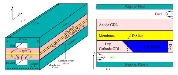
**Figure 1:** (Left) A 3D view of a straight channel PEM fuel cell showing the membrane, catalyst layers, gas diffusion layers (GDLs), and flow fields. The 1D slice of the cathode GDL is indicated by a dotted line. (Right) An along-the-channel (y-z) slice indicating the development of two-phase regions in the cathode GDL. When unhumified gases are used at the air and fuel inlets, the inlet regions of the GDL are typically dry and two-phase regions form down-stream where the gases are more humid.
