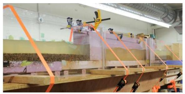
Figure A1. Photograph of the flume setup during one of the runs. Entrance and exit reaches are alluviated, while the canyon reach is mostly clear.
