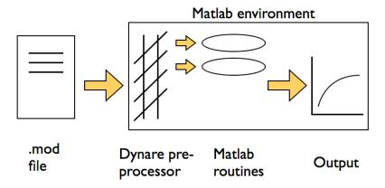
Figure 1.1: The .mod file being read by the Dynare pre-processor, which then calls the relevant Matlab routines to carry out the desired operations and display the results.
