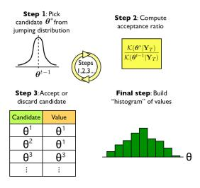
Figure 8.1: The above sketches the Metropolis-Hastings algorithm, used to build the posterior distribution function. Imagine repeating these steps a large number of times, and smoothing the "histogram" such that each "bucket" has infinitely small width.
