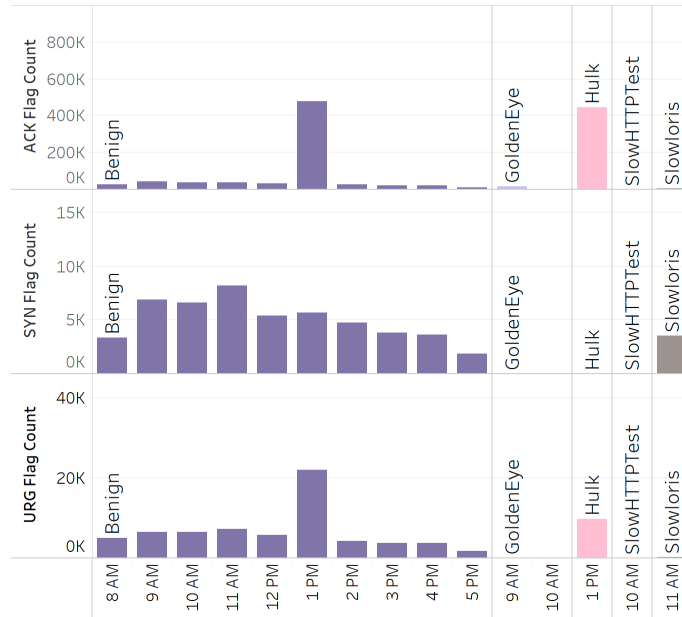
Figure A.7: CSE-CIC-IDS2018: ACK, SYN, and URG flag counts. A large amount of ACK and URG packets is observed at 1 PM.
