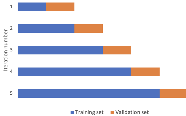
Figure 4.3: Time series split cross validation for k = 5 . In the first iteration, the first subset is used for training while the second subset is used for validation.
