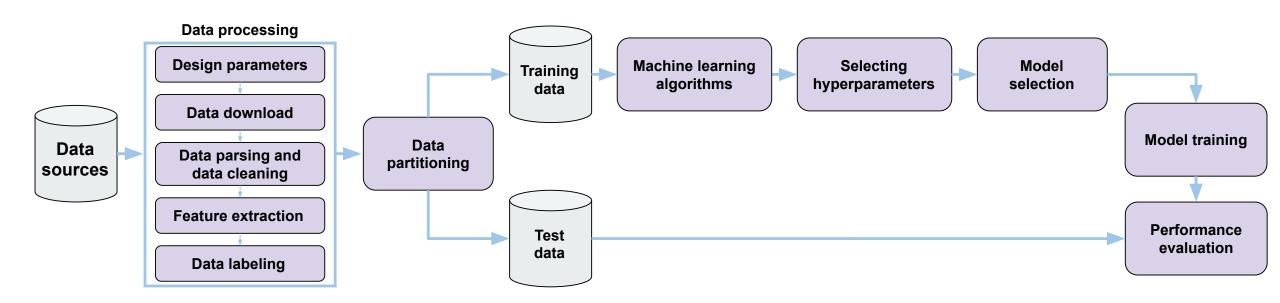
Designing machine learning models to classify network anomalies. The steps include data processing, data partitioning, cross-validation to calculate hyperparameters, model selection and training, and performance evaluation.
