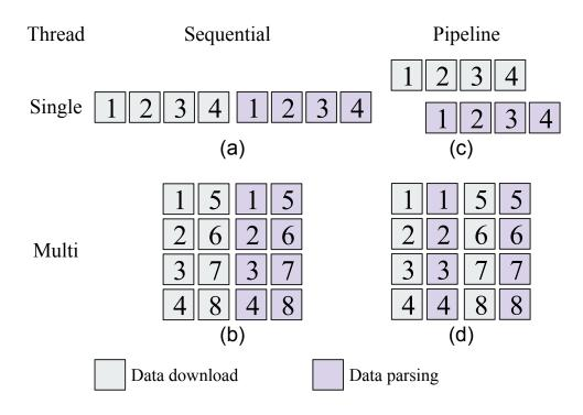
Data download and parsing: (a) data download is completed before parsing; (b) multicore CPUs with data download completed before parsing; (c) data parsing begins before the completion of downloads; (d) simultaneous use of the pipeline and multithreading.
