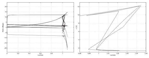
**Fig. 4.** Homotopy paths for the fourteen node voltages of the four-transistor benchmark circuit (left). Closer view of the homotopy path for the voltage at node 10 (right).
