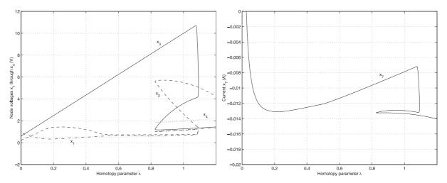
**Fig. 2.** Homotopy paths for the four node voltages  $x_1$  through  $x_4$  (left) and the current  $x_7$ (right) of the Schmitt trigger circuit. The plots show solutions of the homotopy equations vs. the value of the homotopy parameter  $\lambda$ .
