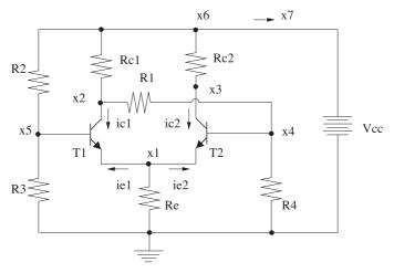
**Fig. 1.** Schmitt trigger circuit whose equations were solved by using homotopy method. Circuits parameters are:  $V_{cc}=10$  V,  $R_1=10$  k $\Omega$ ,  $R_2=5$  k $\Omega$ ,  $R_3=1.25$  k $\Omega$ ,  $R_4=1$  M $\Omega$ ,  $R_{c_1}=1.5$  k $\Omega$ ,  $R_{c_2}=1$  k $\Omega$ , and  $R_e=100$   $\Omega$ . The two bipolar transistors are identical with parameters:  $m_e\alpha_f=m_c\alpha_r=-1.0\times 10^{-16}$  A,  $\alpha_f=0.99$ ,  $\alpha_r=0.5$ , and n=-38.78 1/V.
