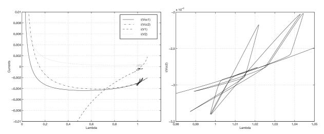
**Fig. 5.** Homotopy paths for the four currents flowing through the four independent voltage sources of the four-transistor benchmark circuit (left). Closer view of the homotopy path for the current flowing through the independent voltage source connected to node number 14 (right).
