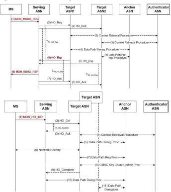
Figure 3. Flow chart of MS-initiated handover: preparation phase (top) and action phase (bottom) [7].
