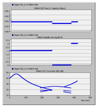
Figure 10. BS\_0 free upload capacity (top), serving BS ID for MS\_0 (middle), and downlink SNRs for MS\_0 (bottom).
