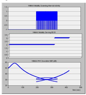
Figure 6. Scanning interval (top), serving BS ID (middle), and downlink SNRs (bottom) for MS 0.
