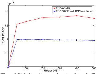
Figure 6. Link throughput as a function of transfer file size. TCP-ADaLR exhibits up to 81% higher link throughput than TCP NewReno.
