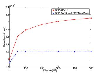
Figure 5. As the transfer file size increases, TCP-ADaLR shows 9%–75% higher TCP throughput compared to TCP NewReno.
