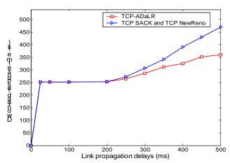
Figure 3. FTP download response time as a function of RTT for a 50 MB transfer file size. For large RTTs, TCP-ADaLR exhibits shorter download response times than TCP NewReno.
