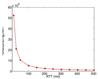
Figure 1. TCP throughput as a function of RTT. TCP throughput decreases as RTT increases.
