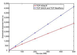
Figure 4. FTP download response time for various transfer file sizes. As the transfer file size increases, TCP-ADaLR shows shorter FTP download response times than TCP NewReno.
