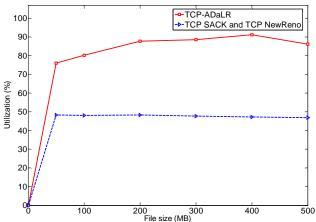
Figure 7. Link utilization as a function of transfer file size. TCP-ADaLR shows 57%–90% higher link utilization than TCP NewReno for the 2 Mb/s link.
