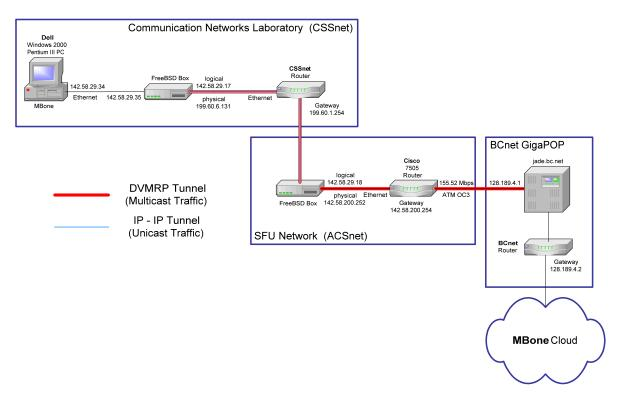
Figure 1: Network setup for the MBone test session in the Communication Networks Laboratory at SFU.
