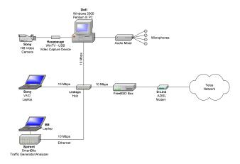
Figure 4: The audio/video and measurement equipment setup for the live MBone webcast session.
