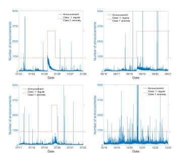
Fig. 1. Number of BGP announcements in Slammer (top left), Nimda (top right), Code Red I (bottom left), and regular RIPE (bottom right) traffic.
