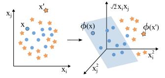
Fig. 3. Illustration of SVM using the nonlinear kernel function  $k(\mathbf{x}_n, \mathbf{x}_m) = \langle \mathbf{x}_n, \mathbf{x}_m \rangle^2$ . View in the three-dimensional space shows a hyperplane dividing regular (circles) and anomalous (stars) data points.
