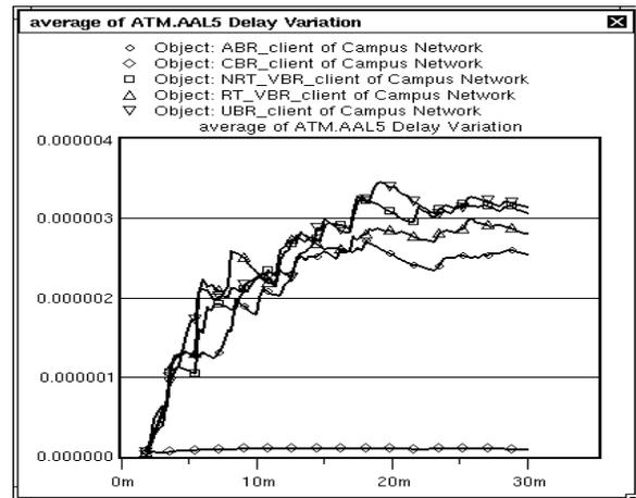
Figure 9. Average delay jitter for different clients of the network shown in Fig. 5.
