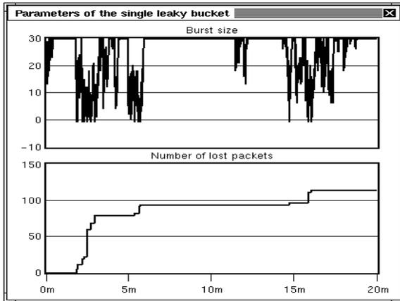
Figure 12. Single leaky bucket: Burst size (cells) allowed into the network (top). Number of lost cells (bottom).
