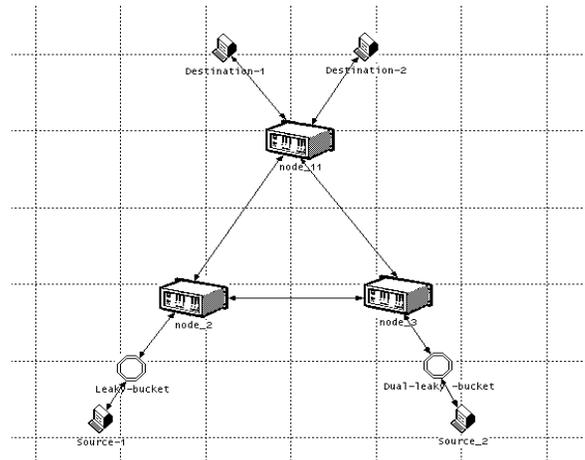
Figure 11. ATM network model. The model consists of a CBR and a VBR ATM source, three ATM switches, and two destinations. A leaky bucket process model is used for each source.
