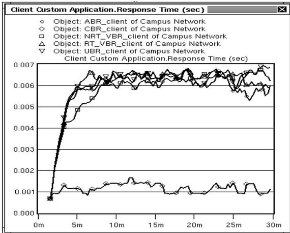
Figure 7. Response time (sec) for each client of Fig. 5. This is the elapsed time between sending a request packet to the server and receiving a response from it.
