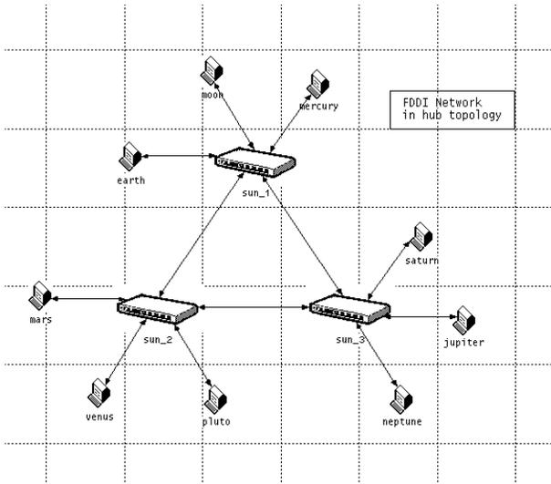
Figure 1. FDDI hub configuration. The network consists of three concentrators (FDDI hubs) and nine stations. The concentrators are connected with FDDI duplex links in a dual-ring topology. The stations are attached to the ring via concentrators, creating a hub topology.
