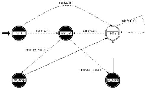
Figure 10. State transition diagram of the leaky bucket process model.
