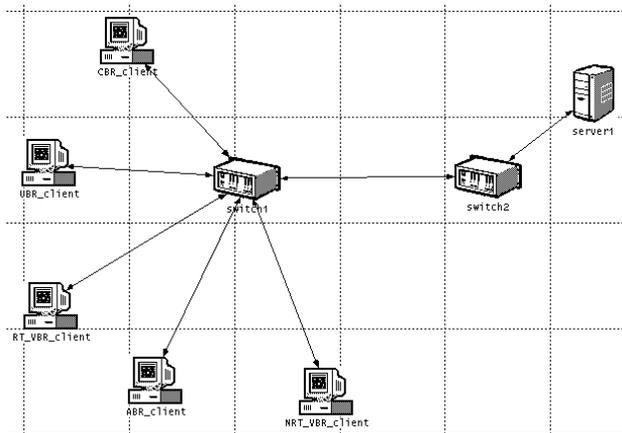
Figure 5. ATM client-server network consisting of two switches, an ATM server, and five clients requesting five distinct ATM service categories.
