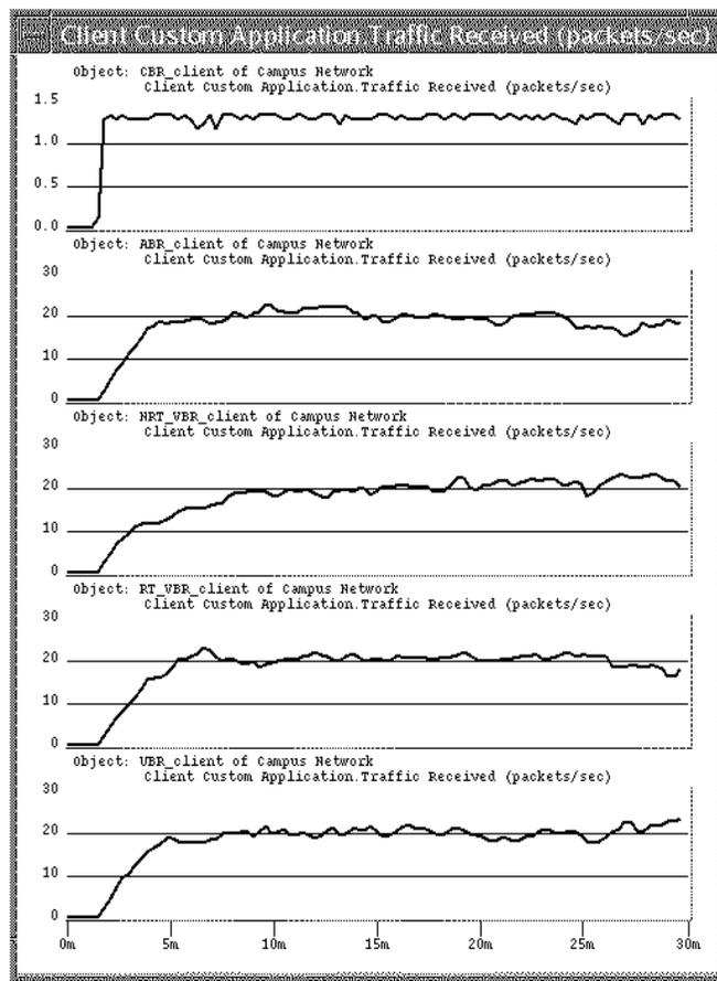
Figure 6. Traffic received (packets/sec) by CBR, ABR, NRT\_VBR, RT\_VBR, and UBR clients (top to bottom) from the server in the network shown in Fig. 5.
