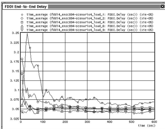
Figure 2. FDDI end-to-end delay (sec) plots, with traffic load as a parameter. Load, mean number of frames sent by the source, according to an exponential distribution, was varied from 1 to 100 packets per second.
