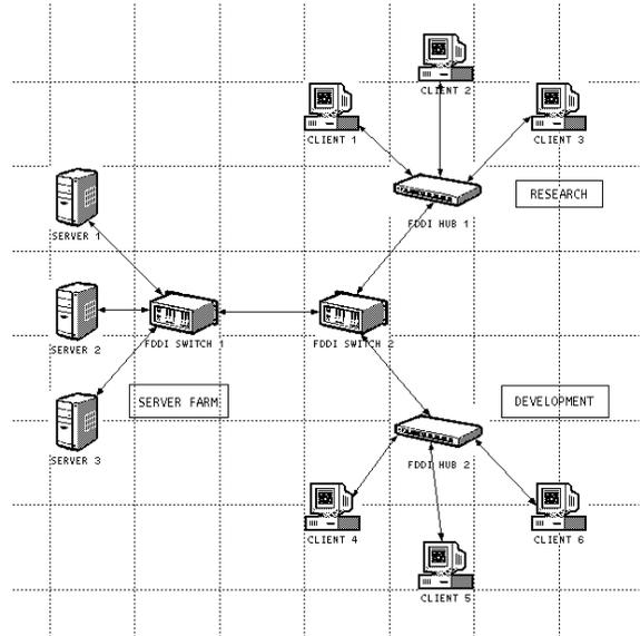
Figure 3. FDDI client-server configuration. This network topology is suitable for applications such as FTP. Clients are connected to the network via FDDI hubs. Hubs and servers at different locations are connected via two FDDI switches.
