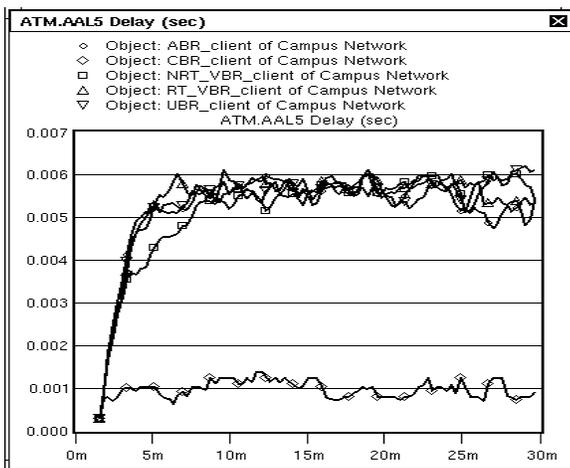
Figure 8. The propagation delay (sec) of packets from each client to the server shown in Fig. 5.
