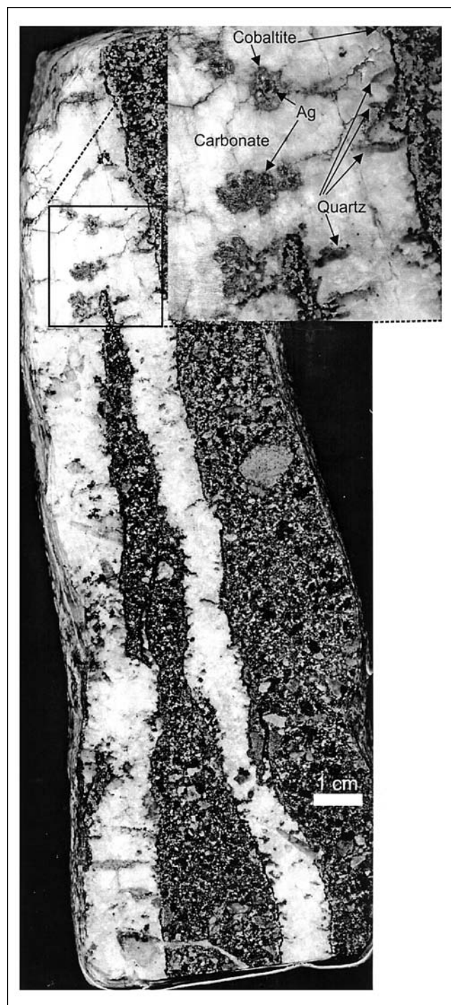
Fig. 5. Bifurcating vein from the Pan Silver mine, showing the typical carbonate-arsenide-Ag assemblage, with quartz crystals and chlorite present on the vein walls.
