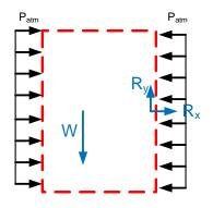
Body force in the y direction is denoted as W. Since we are looking for horizontal forces, we write the x component of the steady flow momentum equation
