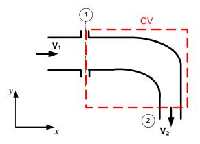
Note that we have several surface forces:  $P_1$  on area  $A_1$  at point 1 and atmospheric pressure,  $P_{atm}$  everywhere else. The exit section 2, is a free jet and so pressure is ambient pressure. We can simplify this problem by subtracting  $P_{atm}$  from the entire surface. Then, final results will be in gage pressure. Force diagram of the elbow is shown as below
