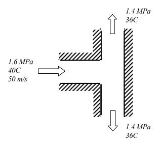
**5-157** The mass flow rate of a compressed air line is divided into two equal streams by a T-fitting in the line. The velocity of the air at the outlets and the rate of change of flow energy (flow power) across the T-fitting are to be determined.
