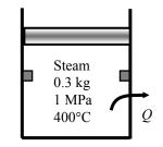
**5-11** Saturated water vapor in a cylinder is heated at constant pressure until its temperature rises to a specified value. The boundary work done during this process is to be determined.
