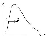
**5-40 CD EES** A cylinder equipped with an external spring is initially filled with steam at a specified state. Heat is transferred to the steam, and both the temperature and pressure rise. The final temperature, the boundary work done by the steam, and the amount of heat transfer are to be determined, and the process is to be shown on a P-v diagram.
