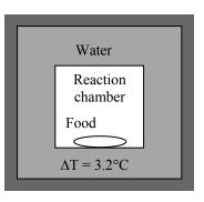
To make a rough estimate of the error involved in neglecting the thermal energy stored in the reaction chamber, we treat the entire mass within the chamber as air and determine the change in sensible internal energy:
