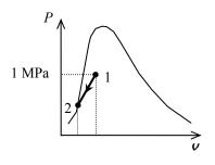
Since this is a linear process, the work done is equal to the area under the process line 1-2:
