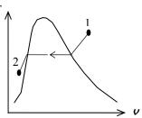
**5-38E** A cylinder contains water initially at a specified state. The water is heated at constant pressure. The final temperature of the water is to be determined, and the process is to be shown on a T - v diagram.
