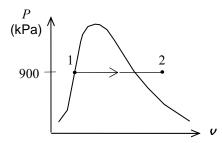
**5-13 EES** Problem 5-12 is reconsidered. The effect of pressure on the work done as the pressure varies from 400 kPa to 1200 kPa is to be investigated. The work done is to be plotted versus the pressure.
