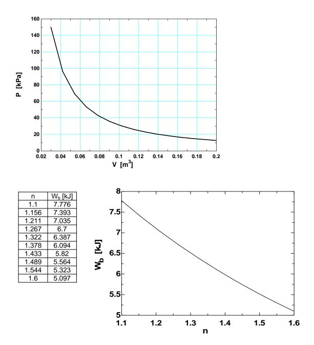
**5-19** Nitrogen gas in a cylinder is compressed polytropically until the temperature rises to a specified value. The boundary work done during this process is to be determined.
