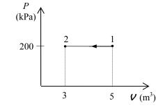
5-6 The boundary work done during the process shown in the figure is to be determined.
