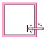
**5-33** Motor oil is contained in a rigid container that is equipped with a stirring device. The rate of specific energy increase is to be determined.
