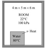
**5-117** A room is to be heated by 1 ton of hot water contained in a tank placed in the room. The minimum initial temperature of the water is to be determined if it to meet the heating requirements of this room for a 25-h period.
