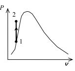
5-103 The boundary work expression during a polytropic process of an ideal gas is to be derived.
