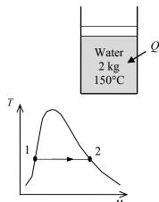
**5-45** A saturated water mixture contained in a spring-loaded piston-cylinder device is heated until the pressure and volume rise to specified values. The heat transfer and the work done are to be determined.
