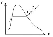
**5-39** A cylinder is initially filled with saturated liquid water at a specified pressure. The water is heated electrically as it is stirred by a paddle-wheel at constant pressure. The voltage of the current source is to be determined, and the process is to be shown on a P-v diagram.
