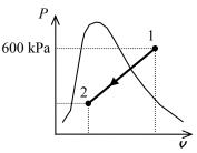
**5-47E** Saturated R-134a vapor is condensed at constant pressure to a saturated liquid in a piston-cylinder device. The heat transfer and the work done are to be determined.
