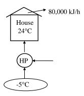
**7-103** A heat pump maintains a house at a specified temperature. The rate of heat loss of the house and the power consumption of the heat pump are given. It is to be determined if this heat pump can do the job.
