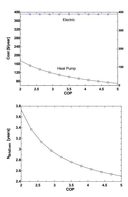
**7-141** A home owner is to choose between a high-efficiency natural gas furnace and a ground-source heat pump. The system with the lower energy cost is to be determined.
