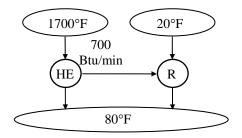
The rate of heat removal from the refrigerated space will be a maximum if a Carnot refrigerator is used. The COP of the Carnot refrigerator is
