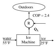
**7-47** The COP and the power consumption of a refrigerator are given. The time it will take to cool 5 watermelons is to be determined.
