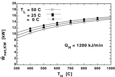
**7-82E** The sink temperature of a Carnot heat engine, the rate of heat rejection, and the thermal efficiency are given. The power output of the engine and the source temperature are to be determined.
