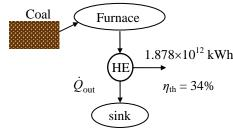
**7-26** The projected power needs of the United States is to be met by building inexpensive but inefficient coal plants or by building expensive but efficient IGCC plants. The price of coal that will enable the IGCC plants to recover their cost difference from fuel savings in 5 years is to be determined.
