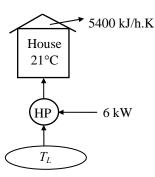
**7-108** A heat pump maintains a house at a specified temperature in winter. The maximum COPs of the heat pump for different outdoor temperatures are to be determined.
