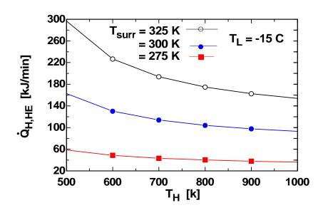
**7-134** Half of the work output of a Carnot heat engine is used to drive a Carnot heat pump that is heating a house. The minimum rate of heat supply to the heat engine is to be determined.
