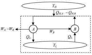
The combined cyclic device then exchanges heat with a reservoir at a single temperature and produces work which is clearly a violation of the Kelvin-Planck statement of the second law. Our assumption the  $COP_A < COP_B$  must then be wrong.
