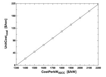
**7-28** The projected power needs of the United States is to be met by building inexpensive but inefficient coal plants or by building expensive but efficient IGCC plants. The price of coal that will enable the IGCC plants to recover their cost difference from fuel savings in 3 years is to be determined.
