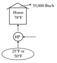
$$COP_{HP,max} = COP_{HP,rev} = \frac{1}{1 - (T_L/T_H)} = \frac{1}{1 - (50 + 460 \text{ R})/(78 + 460 \text{ R})} = 19.2$$
