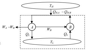
The combined cyclic device then exchanges heat with a reservoir at a single temperature and produces work which is clearly a violation of the Kelvin-Planck statement of the second law. Our assumption the  $COP_B > COP_A$  must then be wrong.
