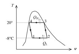
since the enthalpy of vaporization  $h_{fg}$  at a given T or P represents the amount of heat transfer per unit mass as a substance is converted from saturated liquid to saturated vapor at that T or P. Therefore, the fraction of mass that vaporized during heat addition process is
