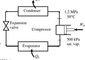
$$\dot{m}_R = \frac{\dot{V}_1}{v_1} = \frac{100 \text{ L/min} \left(\frac{1 \text{ m}^3}{1000 \text{ L}}\right) \left(\frac{1 \text{ min}}{60 \text{ s}}\right)}{0.04112 \text{ m}^3/\text{kg}} = 0.04053 \text{ kg/s}$$
