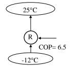
**7-101E** An air-conditioning system maintains a house at a specified temperature. The rate of heat gain of the house and the rate of internal heat generation are given. The maximum power input required is to be determined.
