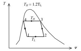
**7-126 EES** Problem 7-125 is reconsidered. The effect of the net work input on the minimum pressure as the work input varies from 10 kJ to 30 kJ is to be investigated. The minimum pressure in the refrigeration cycle is to be plotted as a function of net work input.
