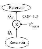
**7-45** The COP and the work input of a heat pump are given. The heat transferred to and from this heat pump are to be determined.
