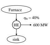
**7-18** The heat input and thermal efficiency of a heat engine are given. The work output of the heat engine is to be determined.
