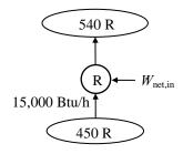
**7-105** The COP of a completely reversible refrigerator as a function of the temperature of the sink is to be calculated and plotted.
