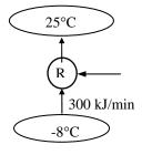
**7-99** The refrigerated space temperature, the COP, and the power input of a Carnot refrigerator are given. The rate of heat removal from the refrigerated space and its temperature are to be determined.
