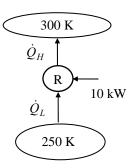
**7-98** The refrigerated space and the environment temperatures for a refrigerator and the rate of heat removal from the refrigerated space are given. The minimum power input required is to be determined.
