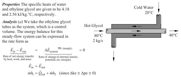
$$\dot{Q}_{\rm out} = \dot{m}c_p(T_1 - T_2)$$
