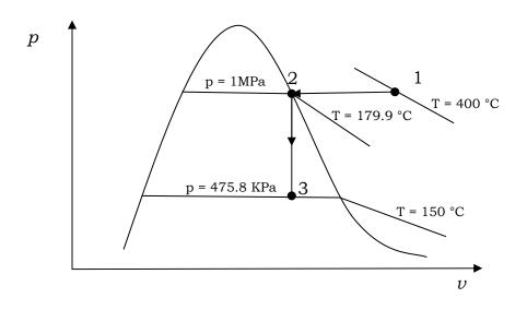
Since the temperature at state 1,  $T_1 = 400^{\circ}C$ , is greater than the saturation temperature corresponding to  $P_1 = 1 MPa$ : 179.9 °C, state 1 is located in the superheated region.
