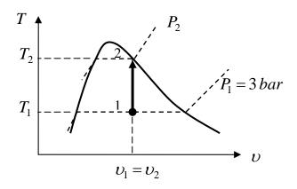
For each state, two independent properties are needed. At initial state (1), the pressure and quality are known. Since 3 bar = 300 kPa, from Table A-5:
