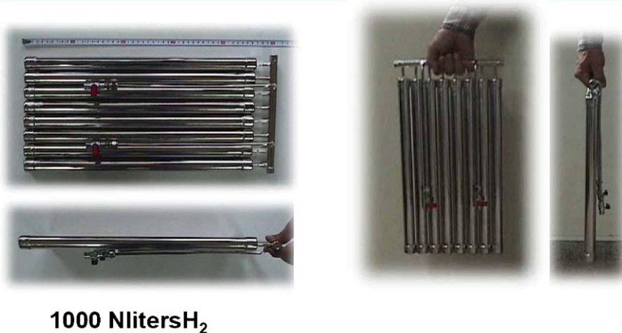
Fig. 6. Air/water-cooled multi-tubular metal hydride storage units [6].
