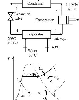
(b) The rate of heat absorbed from the geothermal water in the evaporator is
