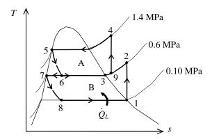
$$\begin{split} \dot{E}_{\rm in} - \dot{E}_{\rm out} &= \Delta \dot{E}_{\rm system} \\ \dot{E}_{\rm in} &= \dot{E}_{\rm out} \\ \sum \dot{m}_e h_e &= \sum \dot{m}_i h_i \\ (1)h_9 &= x_6 h_3 + (1 - x_6)h_2 \\ h_9 &= (0.2527)(262.40) + (1 - 0.2527)(271.40) = 269.13 \text{ kJ/kg} \\ \end{split}$$
