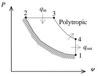
$$T_4 = T_3 \left(\frac{\mathbf{V}_3}{\mathbf{V}_4}\right)^{n-1} = T_3 \left(\frac{2.265\mathbf{V}_2}{\mathbf{V}_4}\right)^{n-1} = T_3 \left(\frac{2.265}{r}\right)^{n-1} = \left(2200 \text{ K}\right) \left(\frac{2.265}{20}\right)^{0.35} = 1026 \text{ K}$$
