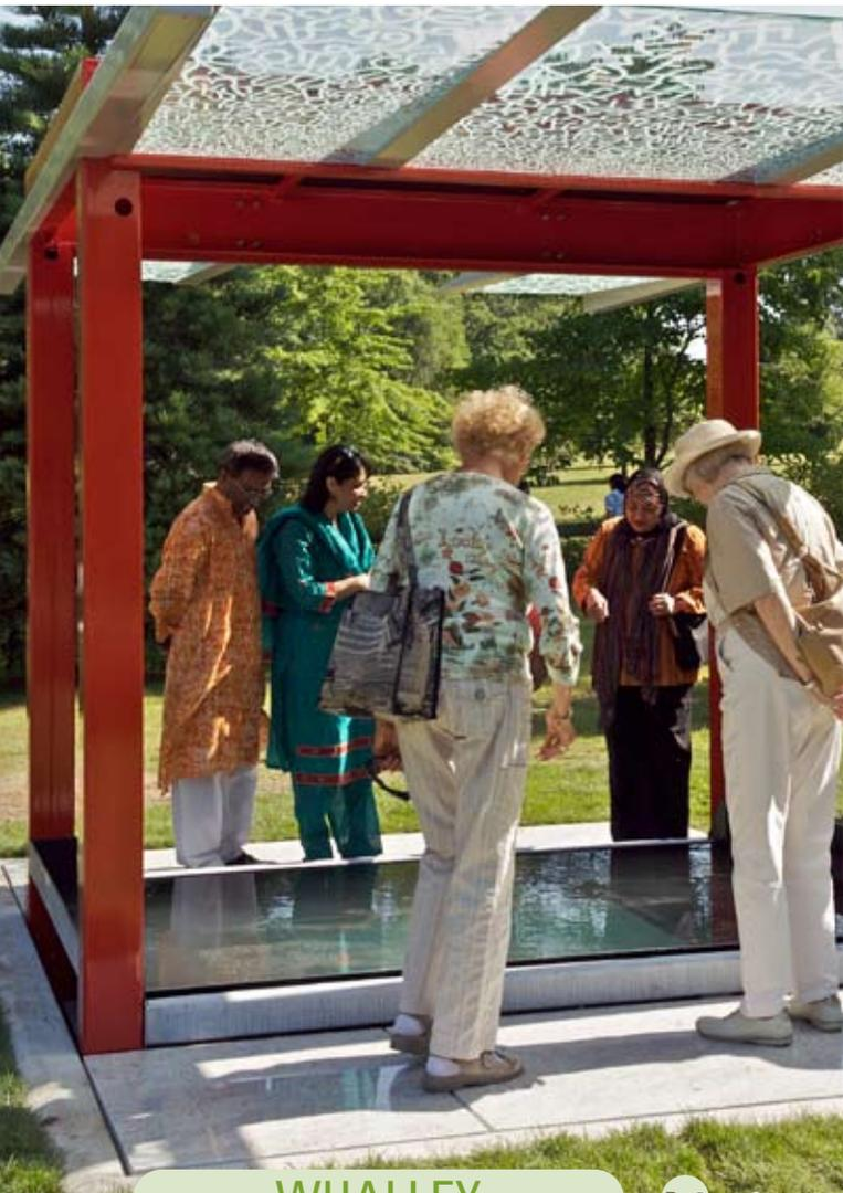
The structure is a self-enclosed fountain, with rain curtains and a reflective pool. A mirror on the underside of the roof reflects the pool and visitors, creating a visual texture and interaction with the structure.
