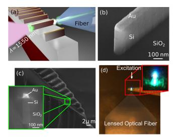
FIG. 3 (color online). (a) Schematic depiction of the conceived device, excitation scheme, and observed visible emission. (b) SEM of a single nanoplasmonic waveguide before deposition of a SiO<sub>2</sub> cladding. (c) SEM of several nanoplasmonic waveguides fabricated on a narrow beam. A close-up of the cross-sectional geometry of the waveguide end facet is shown in the inset. (d) Optical microscope image of visible light emission from the nanoplasmonic waveguides.
