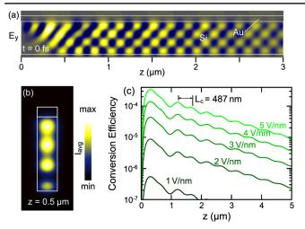
FIG. 2 (color online). (a) Time snapshot of the  $3\omega E_y$  electric field at the fundamental pulse peak arrival. (b) Time-averaged intensity distribution of the  $3\omega$  radiation at  $z = 0.5 \ \mu$ m. (c) Third-harmonic conversion efficiency along the waveguide z axis for peak electric fields of  $E_{\text{neak}}^{\omega} = 1, 2, 3, 4$ , and 5 V/nm.
