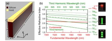
FIG. 1 (color online). (a) Schematic depiction of the siliconbased nanoplasmonic waveguide. (b) Mode dispersion curves for the fundamental and  $3\omega$  wavelengths. Time-averaged intensity distributions (|I|) for three waveguide modes are shown on the right-hand side.
