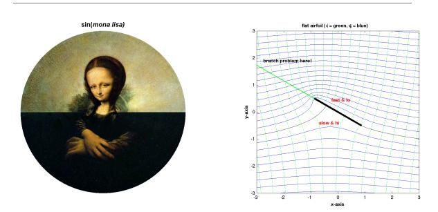
The image on the left is a graphical answer to the complex analysis question, "What is the sine of the Mona Lisa?" It is an example of a conformal map. The image on the right is a visualization of airflow past a flat airfoil (thick black) – the flow follows the blue curves in the direction from left to right. The curves are level contours obtained from a complex-valued function.
