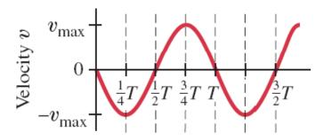
$$v = \frac{dx}{dt} = -\omega A \sin(\omega t + \phi)$$
