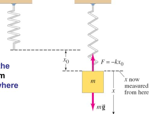
If the spring is hung vertically, the only change is in the equilibrium position, which is at the point where the spring force equals the gravitational force.
