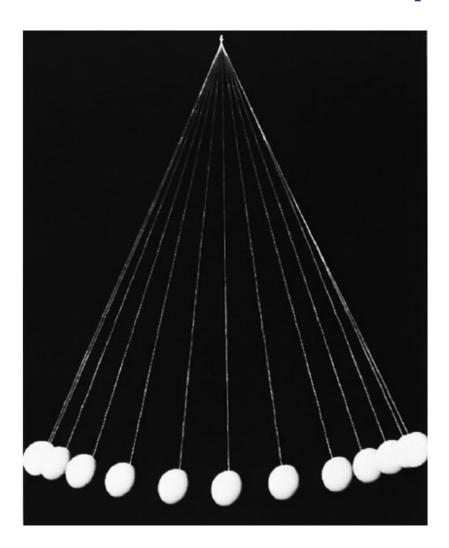
A simple pendulum consists of a mass at the end of a lightweight cord. We assume that the cord does not stretch, and that its mass is negligible.
