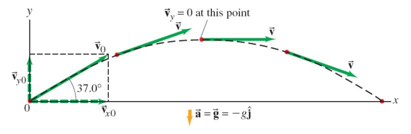
$$v_{x0} = v_0 \cos \theta = 20.0 \cos 37^\circ = 16.0 m/s$$
