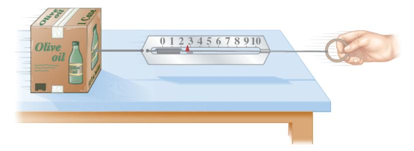
Force is a vector, having both magnitude and direction. The magnitude of a force can be measured using a spring scale.
