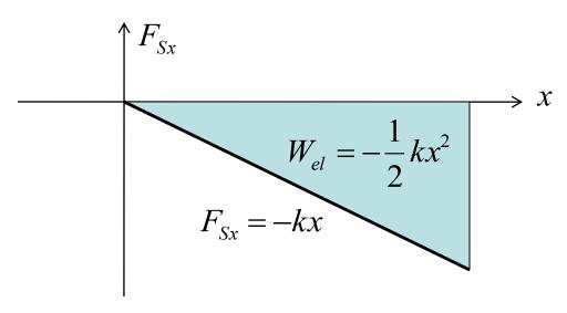
When we stretch (or compress) the spring by x, we raise the potential energy by  $kx^2/2$ .
