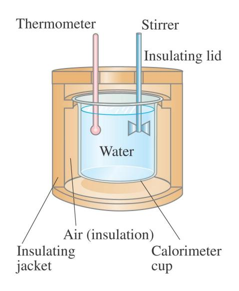
The instrument to the left is a calorimeter, which makes quantitative measurements of heat exchange. A sample is heated to a well-measured high temperature and plunged into the water, and the equilibrium temperature is measured. This gives the specific heat of the sample.
