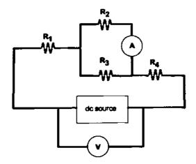
17. [1 pt.] Given that the ammeter in the diagram above reads 2.85A and that  $R_1$ =7.90Ω,  $R_2$ =8.10Ω,  $R_3$ =4.10Ω, and  $R_4$ =5.00Ω, what is the emf of the ideal dc source as indicated by the voltmeter?
