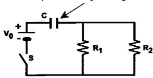
The diagram above depicts an RC-circuit where C=8.40 $\mu$ F,  $R_1$ =11.0 $\Omega$ ,  $R_2$ =18.5 $\Omega$ , and  $V_0$ =20.0V.
