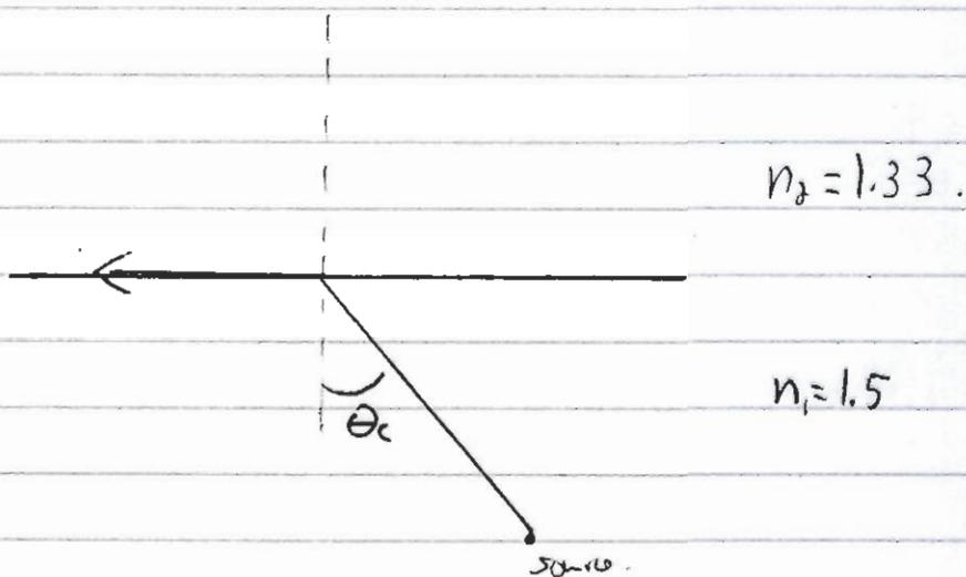
The critical angle occurs when  $\theta_2 = 90^\circ$ , NO Refraction.
