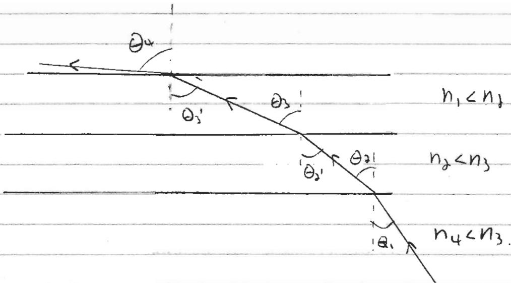
As the above diagram shows, light bends away from the normal if the  $n$  on the refracted side is smaller than the  $n$  on the incident side. One can see this from Snell's law.
