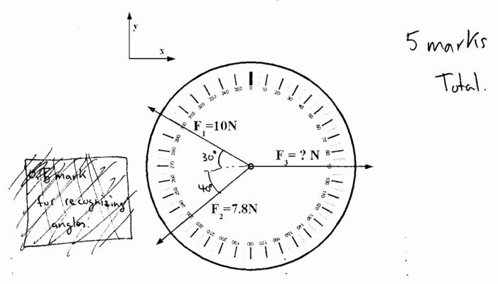
a) Calculate the magnitude of the x and y (using the given coordinate system) component of  $F_1$  and  $F_2$ .  $F_1 = (-10\cos 30 + 10\sin 30 + 10$
