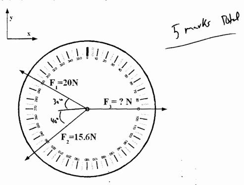
a) Calculate the magnitude of the x and y (using the given coordinate system) component of  $F_1$
