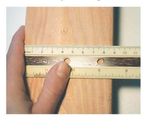
The photograph to the left illustrates this – it would be difficult to measure the width of this board more accurately than ± 1 mm.
