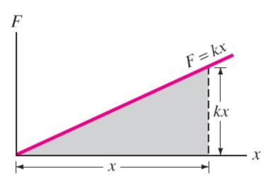
Plot of *F* vs. *x*. Work done is equal to the shaded area.
